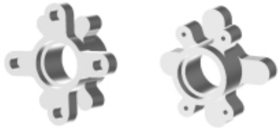
Figure 16. The front hub. Left figure shows the outboard view and the holes for the wheel studs. Right figure shows the inboard view with the holes for the brake rotor.
