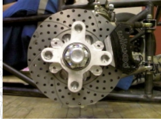
Figure 31. Front right brake system, shown with a modified Wilwood caliper, the rotor, as well as the hub assembly over the spindle bolt.
