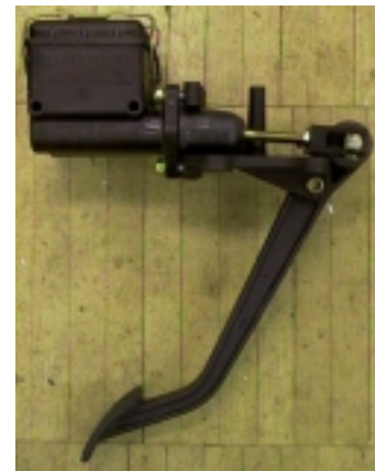
Figure 33. Wilwood pedal assembly, shown with dual master cylinders and balance bar.
