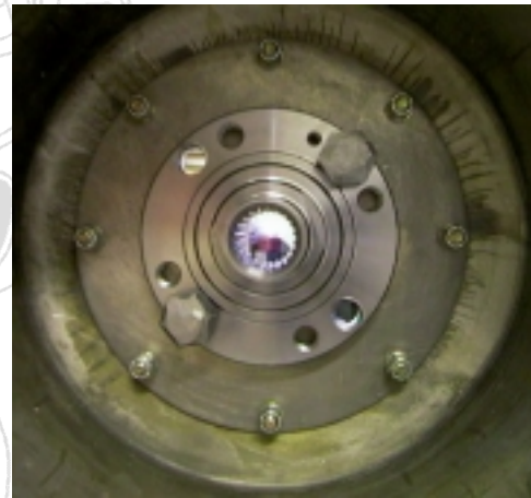
Figure 17. The rear hub, a Volkswagen product, seen from inside a wheel. The hub comes with female splines to fit the outboard constant velocity joint.
