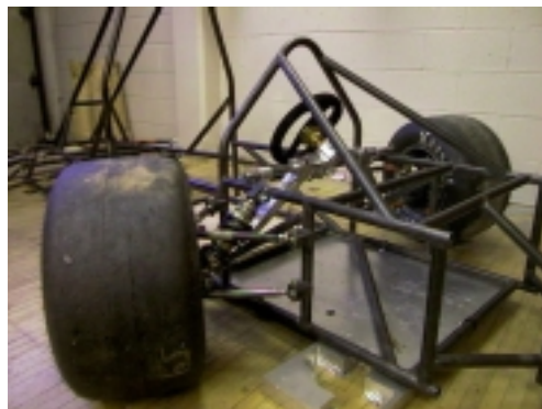
Figure 25. This view of the car clearly shows the Ackermann steering effect that causes the inside wheel to steer more than the outside wheel.
