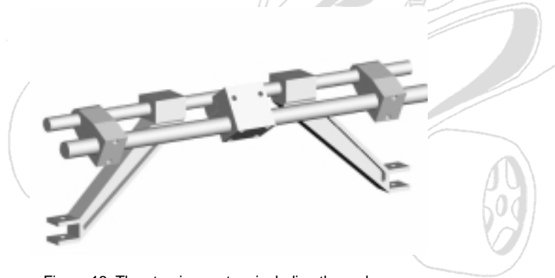
Figure 18. The steering system including the rack, supports and "z-links."
