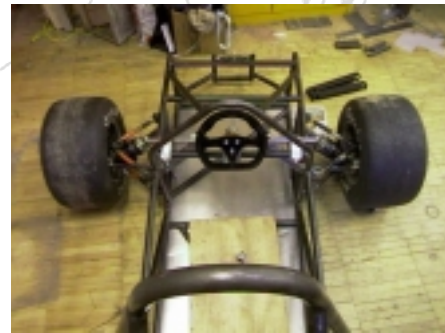
Figure 19. An overhead view of the front axle including the steering system.
