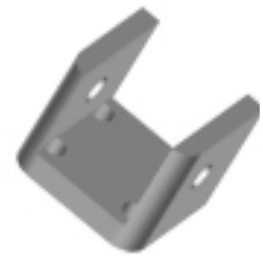
Figure 30. Modular front outer steering track rod attachment to the front upright can be changed to alter steering characteristics without remanufacturing the entire upright.
